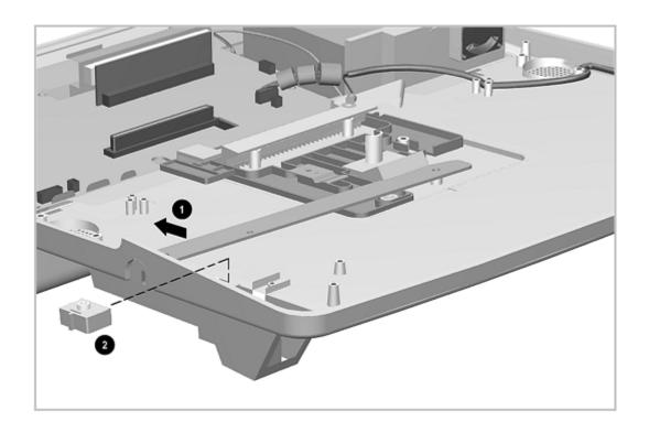
Figure 7-39. Removing the Docking Lever Slider
